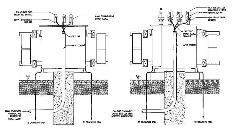
TRANSFORMER LOW VOLTAGE SIDE CABLE TERMINATION SCALE
